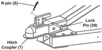
Figure O: Remove R-pin and Lock Pin
